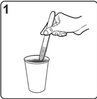
Weigh and pour your material (53/47 ratio by weight) and begin mixing. Mix in a figure-eight motion, scraping both the bottom and sides of the cup. The material will quickly start to thicken, become warm, and will be ready to begin brushing into your mold.
