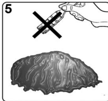
5 Stop brushing the material once it becomes stringy and freezes in place. If you continue brushing, the material could pull away from the silicone mold. At this stage, additional layers of resin may be brushed on if desired.
